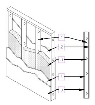
FIGURE 12—FIRE-RESISTANCE-RATED, 1-HOUR, EXTERIOR WALL ASSEMBLY WITH INSULATION IN THE WALL CAVITY. SEE SECTION 4.6.3 FOR ADDITIONAL DETAILS
